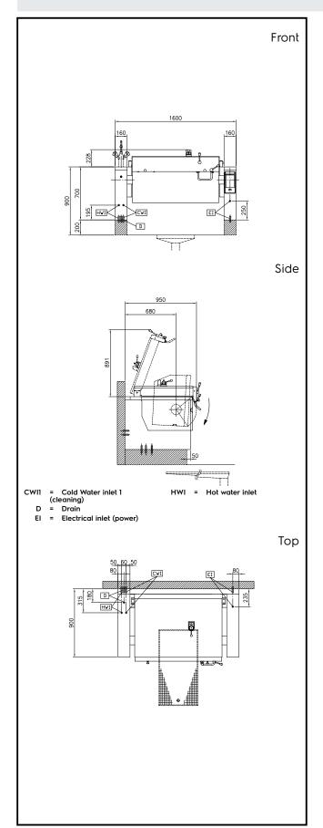
Electric Supply voltage: 400 V/3N ph/50/60 Hz Total Watts: 20.6 kW Installation: FS on concrete base;FS on feet;On base;Standing Type of installation: against wall
